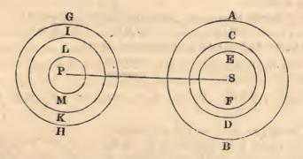
Suppose any number of spheres C D and E F, I K and L M, &c. to be concentric with the spheres A B, G H, respectively; and let C D and I K, E F and L M be homogeneous respectively; then each of these spheres will attract each other with forces  $\alpha^{g}$ .  $\frac{1}{\text{distance}^{2}}$ . Now suppose the original spheres to be made up by the addition and subtraction of similar and homogeneous spheres, each of these spheres attracting each
